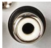
Electrical connector on decoder (Note: Colour is orange, not white as shown)
